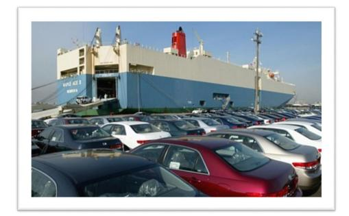
Roll-on/roll-off (RORO or ro-ro) ships are vessels designed to carry wheeled cargo, such as cars, trucks, semi-trailer trucks, trailers, and railroad cars, that are driven on and off the ship on their own wheels or using a platform vehicle, such as a self-propelled modular transporter.
