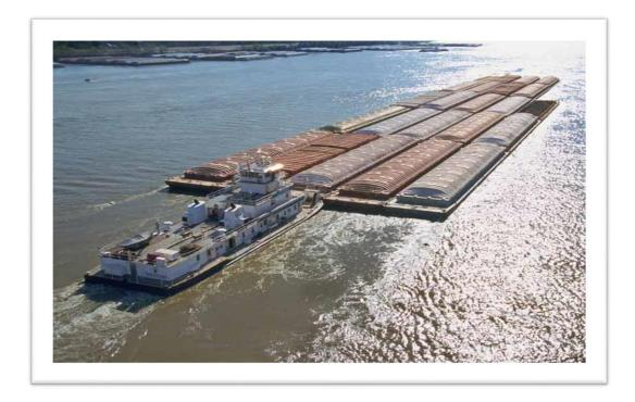
A barge is a flat-bottomed boat, built mainly for river and canal transport of heavy goods. Some barges are not self-propelled and need to be towed or pushed by towboats.
